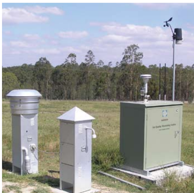
Continuous PM10 dust monitoring unit and High Volume Dust Samplers located along Falbrook Road.
