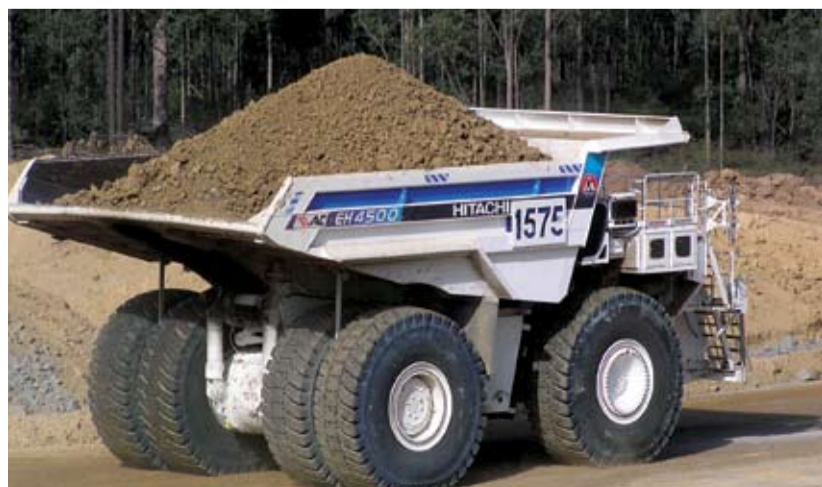
A noise attenuated Hitachi 270mt dump truck hauling overburden to the Mt Owen West Dump.
